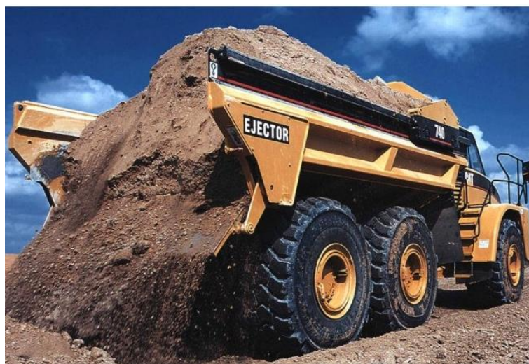
Figure 1 - BELL B50D Ejector Dump Truck with ejector discharge
